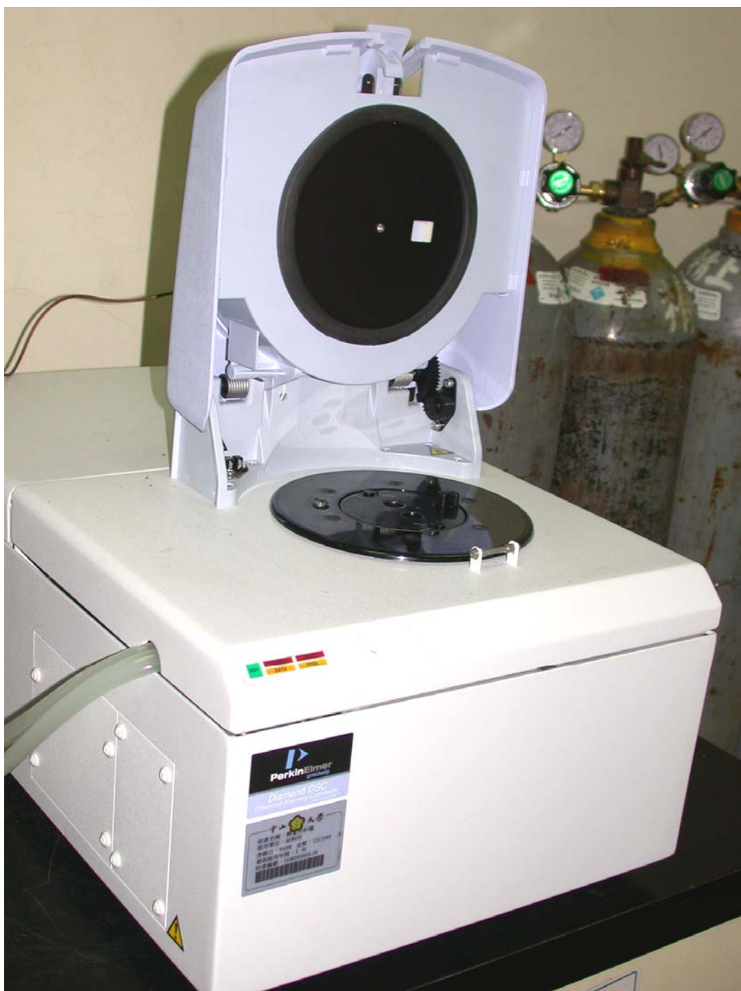
Figure 3.5 The picture of Perkin Elmer Diamond DSC.
