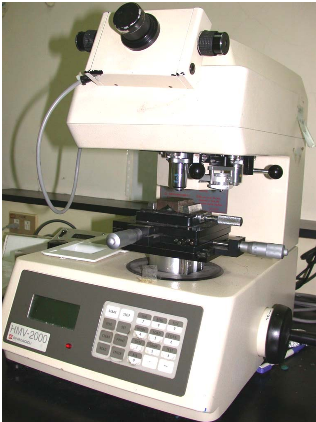
Figure 3.7 The photo of a Shimadzu HMV-2000 Vicker's microhardness tester.
