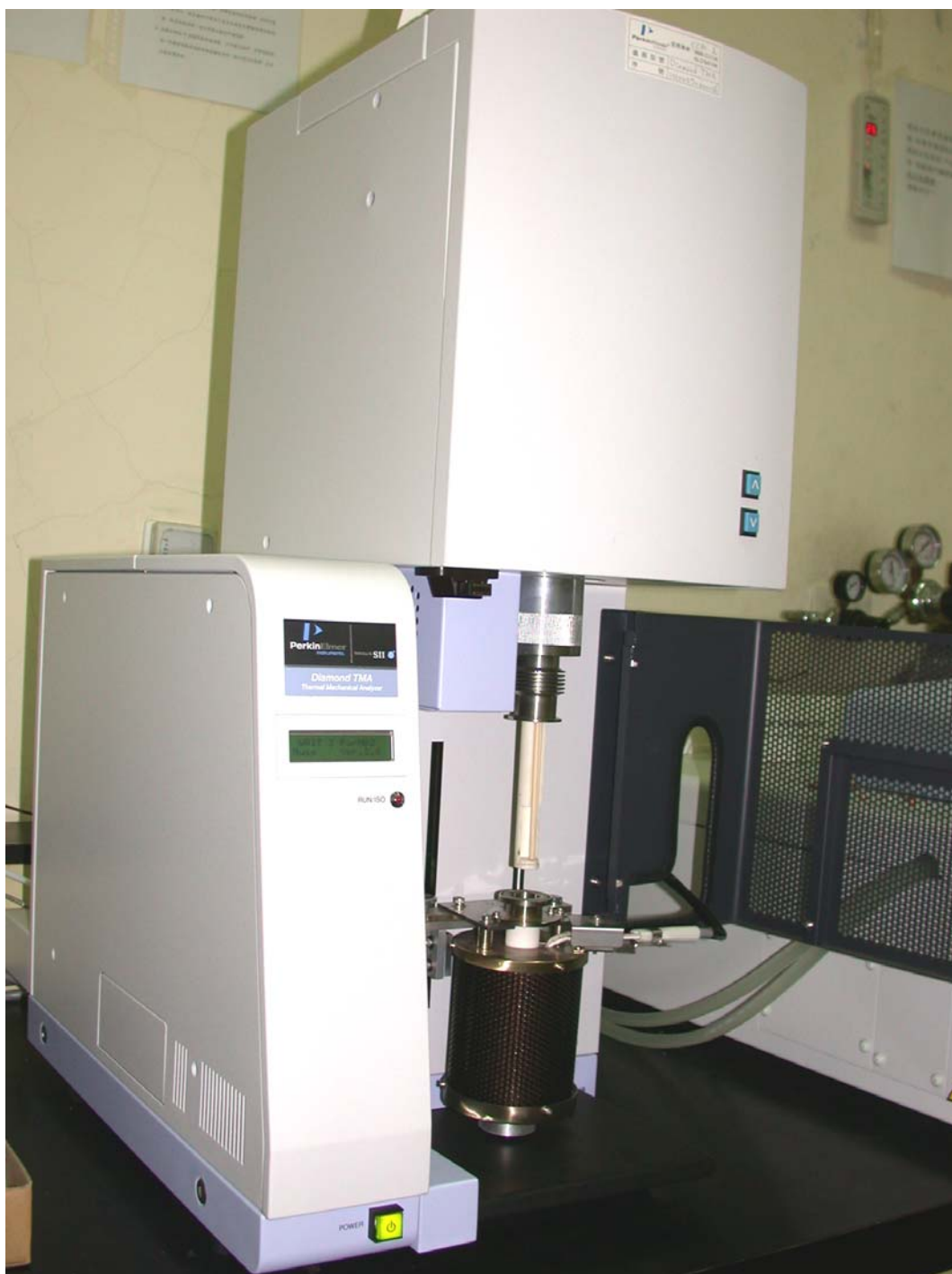
Figure 3.10 The picture of thermomechanical analyzer (TMA 7, Perkin Elmer Diamond)
