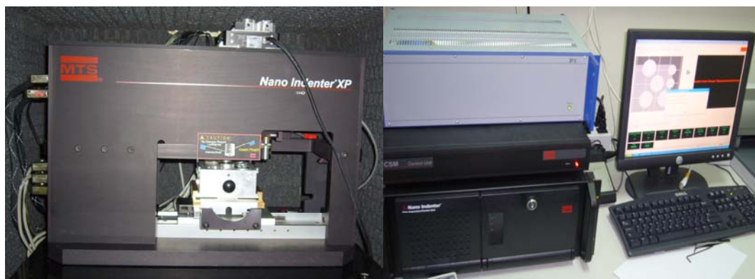
Figure 3.8 The standard Nano Indenter® XP is a complete, turnkey system consisting of the major components illustrated.
