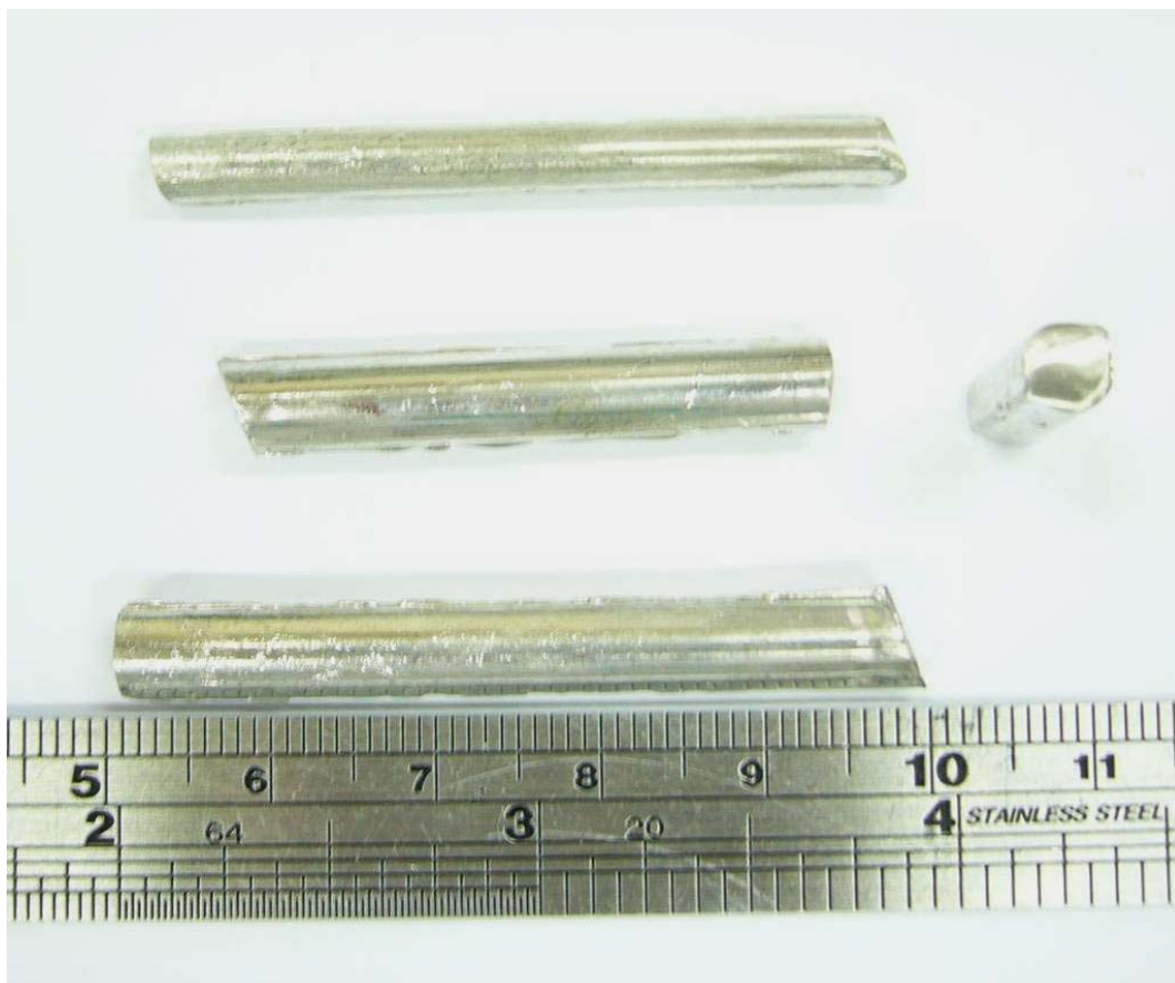
Figure 4.5 The photo showing the surface appearance of injection cast Mg 58 Cu 31 Y 11 alloy samples with different diameters, from 3 and 4 mm.
