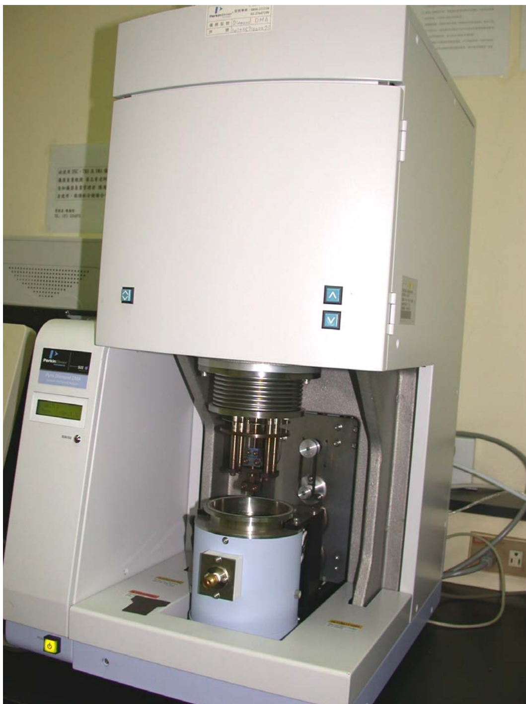
Figure 3.9 The photo of dynamic mechanical analyzer (DMA, Perkin Elmer Diamond DMA)
